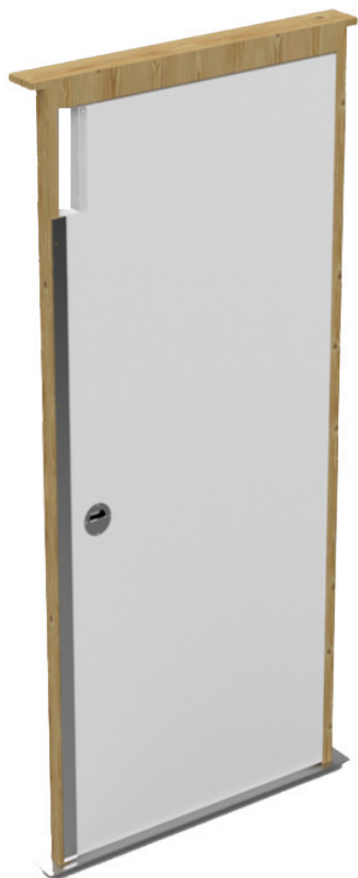
HOISTWAY VIEW WITH 1/8" SHEET-METAL STOPPER
