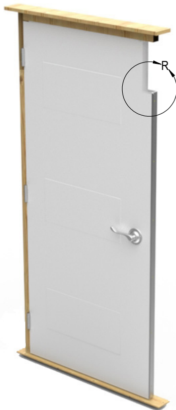
HOUSE VIEW WITH "L" BRACKET STOPPER
