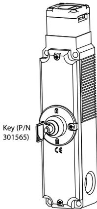
For units with a **GAL lock** or **Prolock**, the door can be opened manually using a special key inserted into the round pin on the front of the lock (Figure 8).
