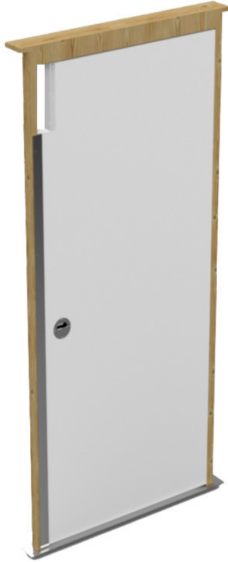
HOISTWAY VIEW WITH 1/8" SHEET-METAL STOPPER
